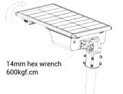
Step 2: A: Put the lamp into the pole, tighten the M10 screw with a torque of 250kGF. cm. B: tighten the M10 nut with a torque of 150kGF. cm (preparation tools:5MM inner hexagon wrench,17mm outer hexagon wrench)
