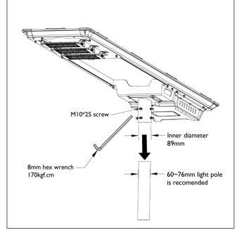
4. Torque 8kgf. Cm locking screw, screwdriver or cross screwdriver to adjust the appropriate irradiation angle of the light source, Rear open switch button.
