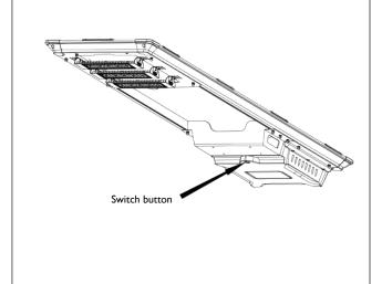
2. Preparation tools: screwdriver or 8mm Allen wrench, socket support, M10\*20 screw 4pcs, socket support, assembly as shown in the following schematic diagram. Pay attention to the vertical installation of lamps with a torque of 250kgf Cm tighten the screws
