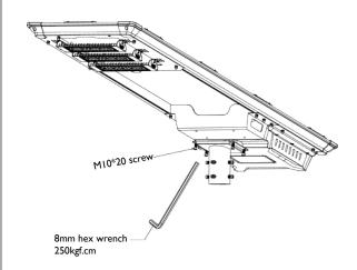
3. Insert the lamp into the lamp pole with a torque of 170kgf Cm tighten screws (prepare M10\*25 screws, 6pcs, screwdriver and 6# Allen wrench).
