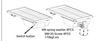
Step 3: Loosen the screws on the universal support and adjust the irradiation Angle of the solar panel. Tighten the screws with a torque of 600kGF. cm and adjust the Angle of -90\*-+90. It is recommended that the installation Angle be 15 degrees (preparation tool :14MM hex wrench).
