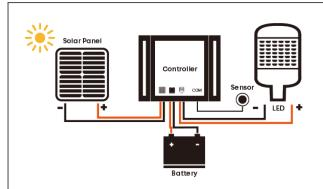
During the day, the solar light shines on the solar panel, generating electric energy, which is controlled by the controller to charge the battery. In the evening, the solar light darkens, when the illumination is 15~25LX, the controller stops charging, and then drives the LED light to turn on. If there is an induction function, the light becomes bright when the induction, and the light becomes dark when there is no induction.
